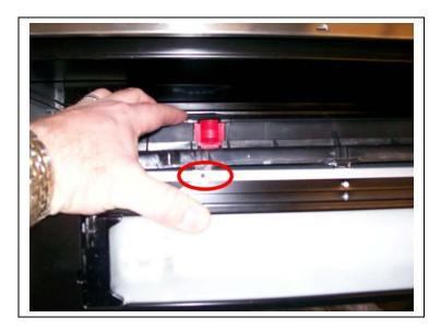
4. Press the front of the charcoal kit down and insert 2 of the screws provided with the charcoal kit into the 2 tabs that are circled in the photo.
