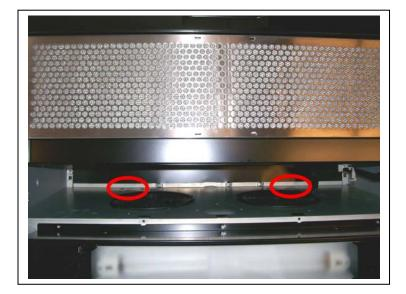
3. Locate the 2 metal tabs inside the hood.Notice the 3 plastic tabs on the charcoal kit.Hook the plastic tabs on the charcoal kit into the 2 metal hoops inside the hood.
